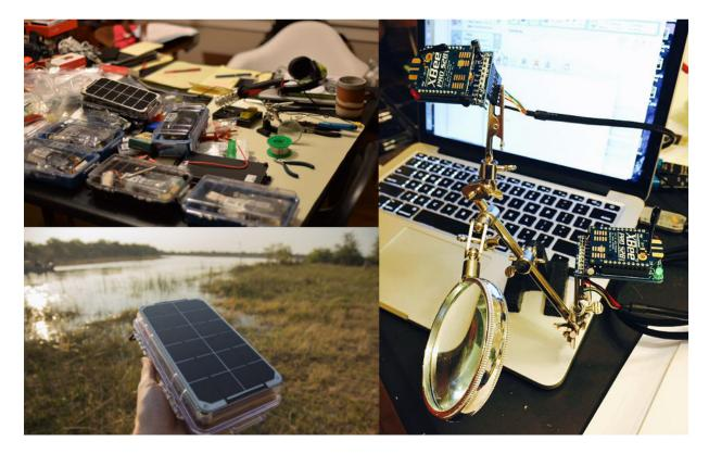
Each of the nodes consist of an <u>Arduino</u>, <u>XBee</u>, and multiple sensors. The XBee ZigBee network makes it possible to connect over long distances since data packets can hop between neighboring nodes until they reach the central coordinator. For power, the remote nodes rely on a solar panel and a 6600 mAh battery.
